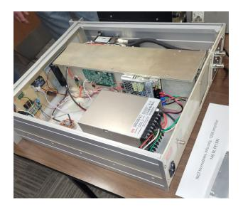
Workmanship Award—222 MHz 250 W power amplifier. This was a collaboration between George, KA3WXV, and Tom, KA3FQS. The project was built in an old traveling wave tube amplifier chassis which provided a nice cooling channel for the amplifier heat spreader. The fabrication was done in the KA3FQS workshop and the amplifier has become a component of the KA3FQS station.
